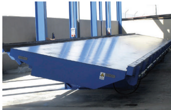
1-rasm. Panel ishlab chiqarish uchun universal rotor vibrostend
