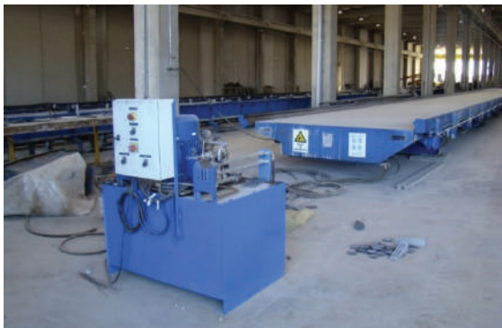
1-rasm. Panel ishlab chiqarish uchun universal rotor vibrostend
